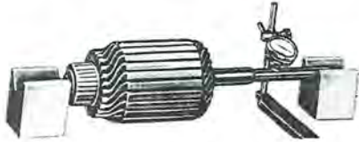
Fig. 15-Checking Armature for Bent Shaft
