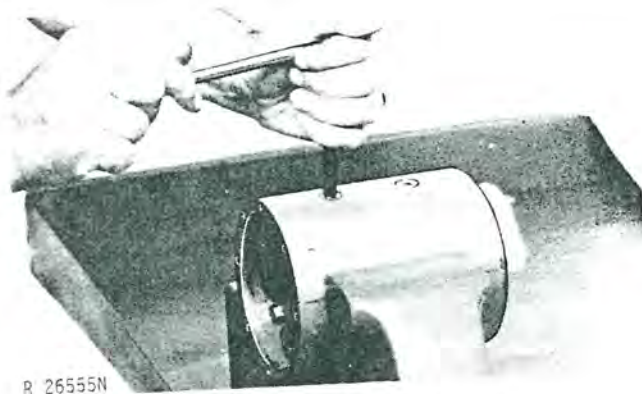
Fig. 9-Removing Pole Shoe Screws
