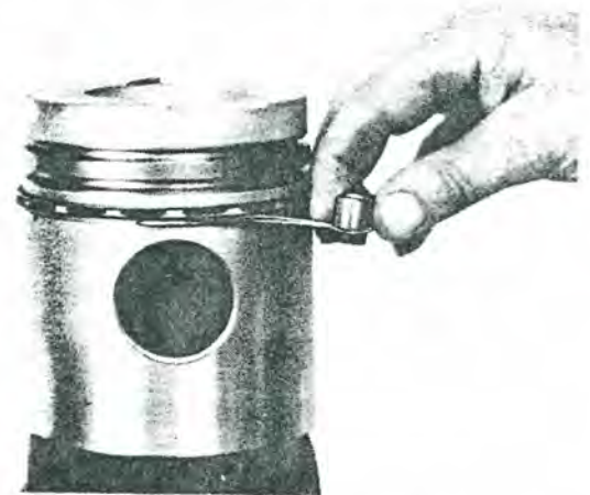
Fig. 5-Checking Oil Control Ring Groove Clearance
