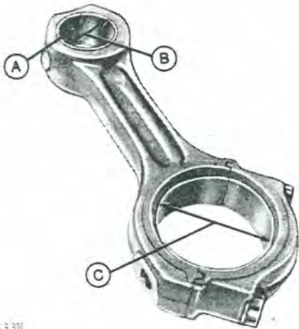
A—Pin Bushing Lubrication Hole B—Pin Bushing Measurement C—Bearing Insert Measurement
