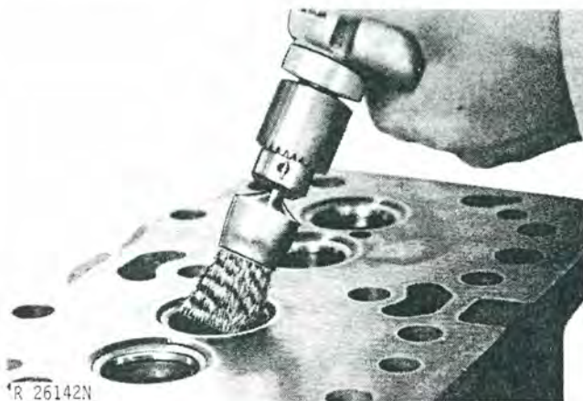
Fig. 16—Cleaning Valve Seats
